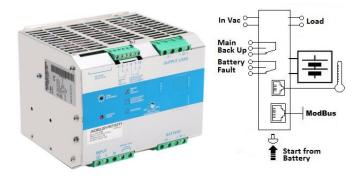
Input: Single-phase 115 – 277 Vac; 500W Output Load: power supply 12 Vdc; 35 A Output Battery: charging 12 Vdc; 35 A
